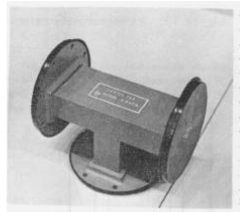
Fig. 24-11. A waveguide "T." (The flanges have plastic end caps to keep the inside clean while the "T" is not being used.)
